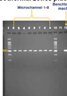
Gel results of PCR products generated from multichannel PCR microchip.
